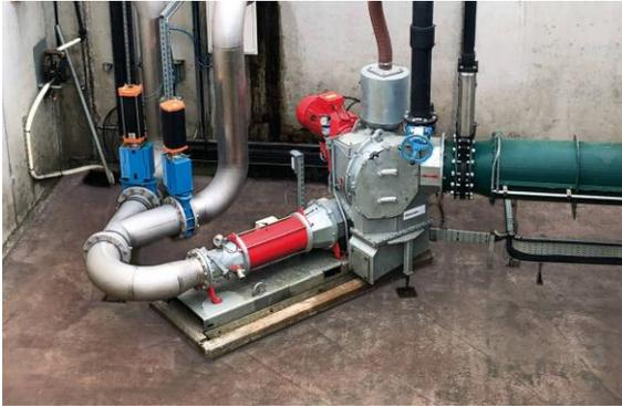
**Image 1:** The universal PreMix solid matter feeder mashes different substrates into a homogeneous organic suspension.
