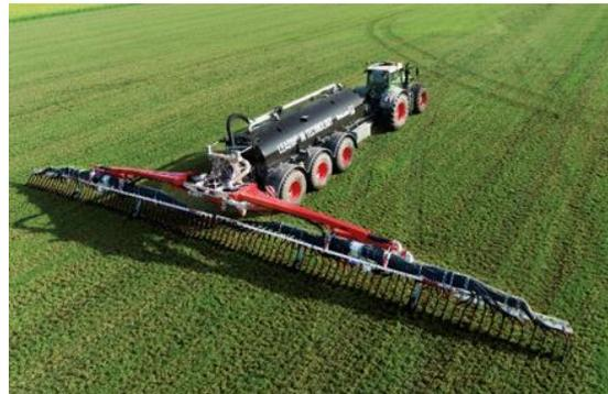
**Image 4:** The BlackBird trailing shoe system with a working width of 24 meters distributes the liquid manure precisely at the plant.
