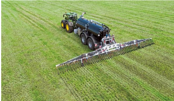
Image 2: In June 2019, Vogelsang launched the trailing shoe linkage “BlackBird” with flow optimised liquid manure discharge on the market.
